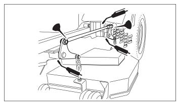
Figure 17. Deck Lift Linkage Pivots
